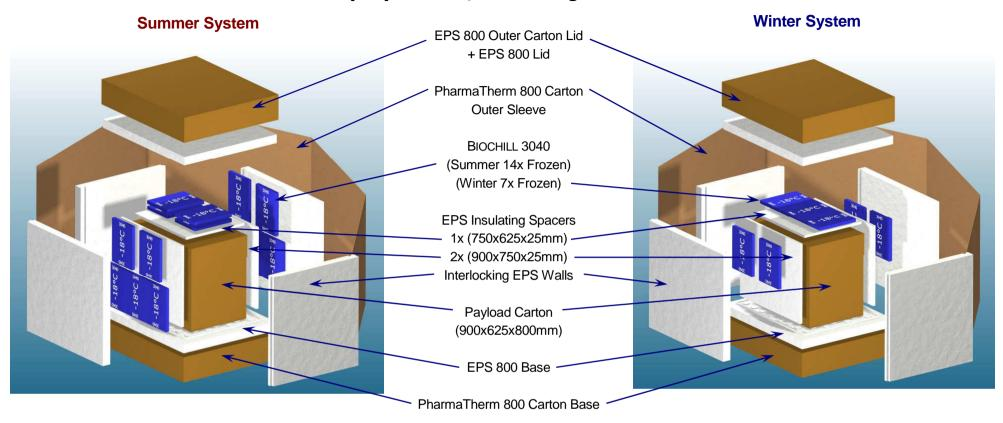
Chilled BIOCHILLs should be conditioned at +5°C for a minimum of 24 hours before use. Frozen BIOCHILLs should be conditioned at -18°C for a minimum of 24 hours and then for approximately 20 minutes at factory ambient +20°C (± 5) before system assembly.
